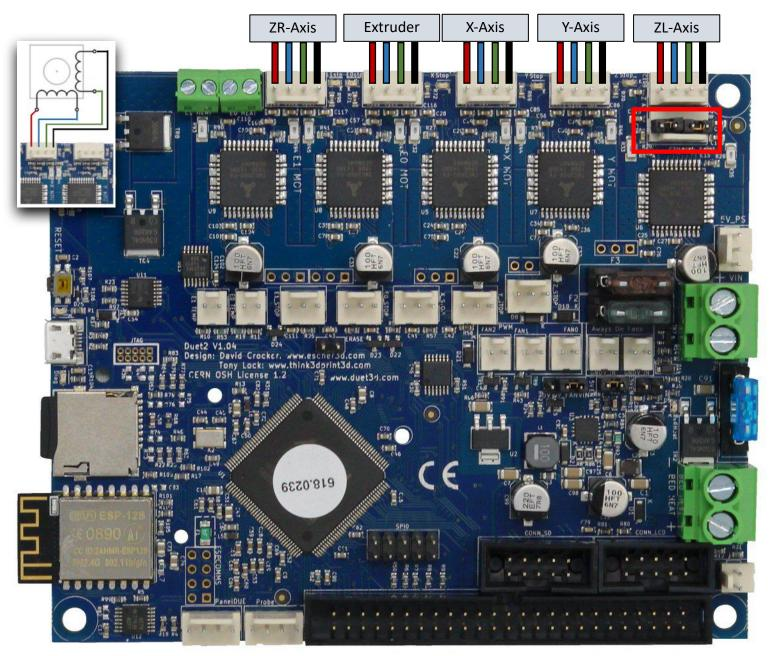
\*Be sure that the supplied jumpers are installed on the ZB connector. Coil 2: Red(-) Blue(+) / Coil 1: Green(+) Black(-)
