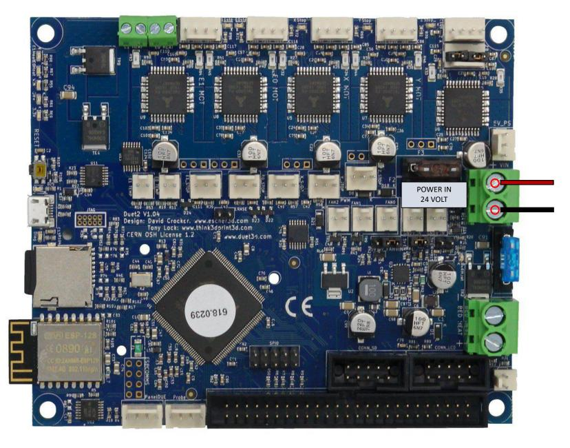
\*Unlike the Einsy RAMBo controller board, the Duet controller only requires 1 set of power cables.
