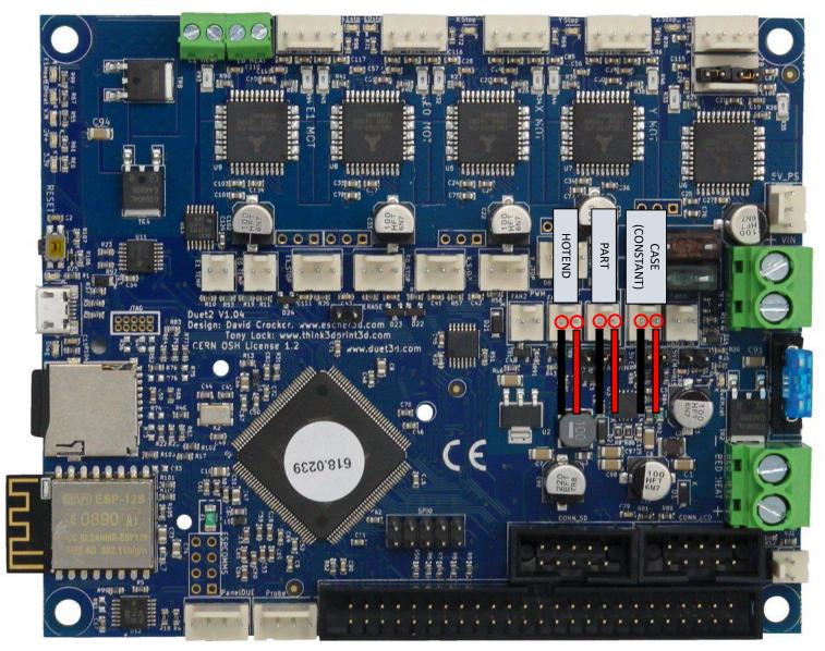
\*The case fan is optional. As shown, the two rightmost connections are constant supplied - always on. The far left (FAN2) connection is available and can be programmed to operate at a defined condition, such as when the MCU or hotend reach a certain temperture. This is beyond the scope of this guide, but information is available in the forums.
