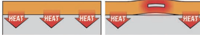
Proper installation ensures good heat flow from the heater to the heat sink
