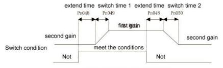
Gain switching sequence diagram
