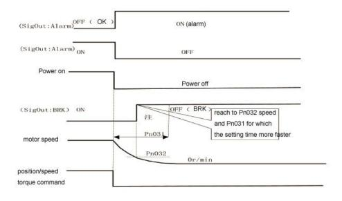
Note 1: when using electromagnetic brake function, servo broken way can make Pn005 must be set to 2
