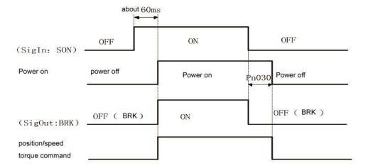
Note 1: when using electromagnetic brake function, servo broken way can make Pn004 must be set to 2.
