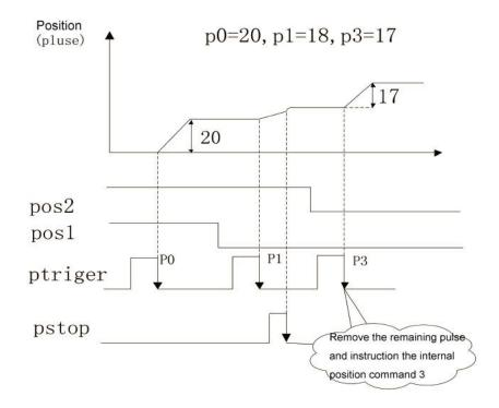
If set Pn118 = 1, want to pause in the process of the position the motor running, when the trigger input port pstop signal, motor speed to stop, when the input port ptriger fire again, the location of the electricity opportunities continue to walk the remaining instructions, the input port pstop trigger issued before the target location, please refer to the following sequence diagram:
