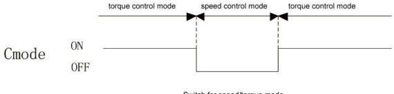
Switch for speed/torque mode
