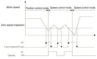
Switch for position/speed control mode
