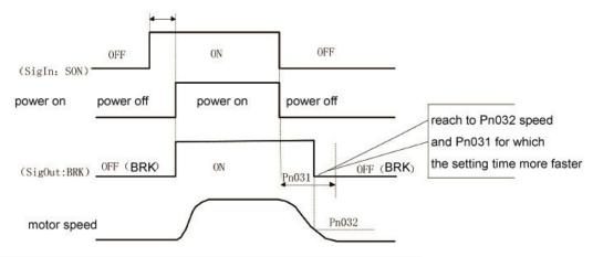
Note 1: when using electromagnetic brake function, servo broken way can make Pn004 must be set to 2
