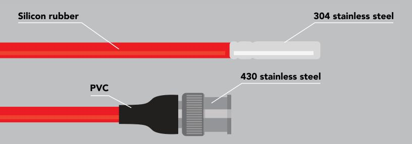
This PT-1000 probe can be *fully submerged* in fresh or salt water, up to the BNC connector *indefinitely*.
