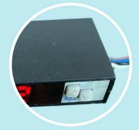
Press the Up key to select the parameter directory to be adjusted for PI, P2, and Np. After selecting the directory, press the Down key to enter the corresponding parameter setting.
