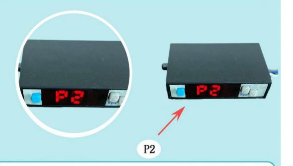
The P2 setting value represents the recovery value, for example, set to -55. When the vacuum value drops from a high value to -55 or below, the Npn signal recovers. There is no need to wait until the vacuum value drops to 0 before the signal is restored.
